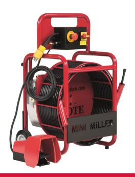
The Mini Miller is a high speed, high torque unit designed for cleaning, descaling, and removing roots in pipes between DN50-100 (2-4") pipes and for cutting/reinstatements in DN50-75 (2-3") pipe. When paired with the Picote Mini Coating Pump it is capable of brush coating in DN50-150 (2-6") pipes as well.
